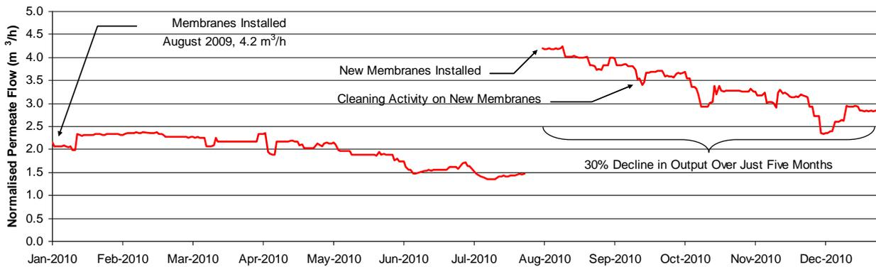
Figure 11 - Normalised Output from Adjacent SWRO Facility 2010
