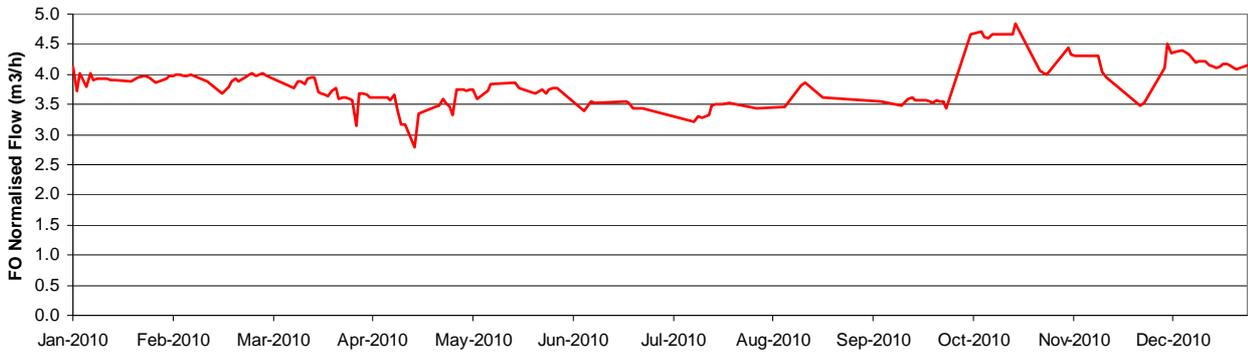
Figure 12 - Normalised Output from FO System 2010
