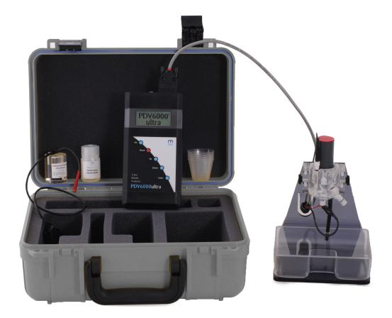
The PDV has been upgraded to allow much improved stand-alone operation and an indication of blank and standard run performance. A larger screen allows simple voltammograms to be shown. The USB connector replaces the serial port. The upgraded product can be run either on 4 x 1.5V AA batteries, or from the mains using the standard 8 - 12V DC transformer.
