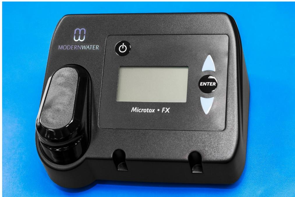
The Microtox FX uses bioluminescence technology to screen for both acute toxicity and microbial contamination. Modern Water's proprietary Microtox technology is considered the industry standard for rapid acute toxicity testing. The test is sensitive to more than 2,700 different and complex compounds with microbial detection levels in drinking water to 100 cfu/ml. Modern Water's Microtox technology has been cited in over 700 peer reviewed independent publications.
