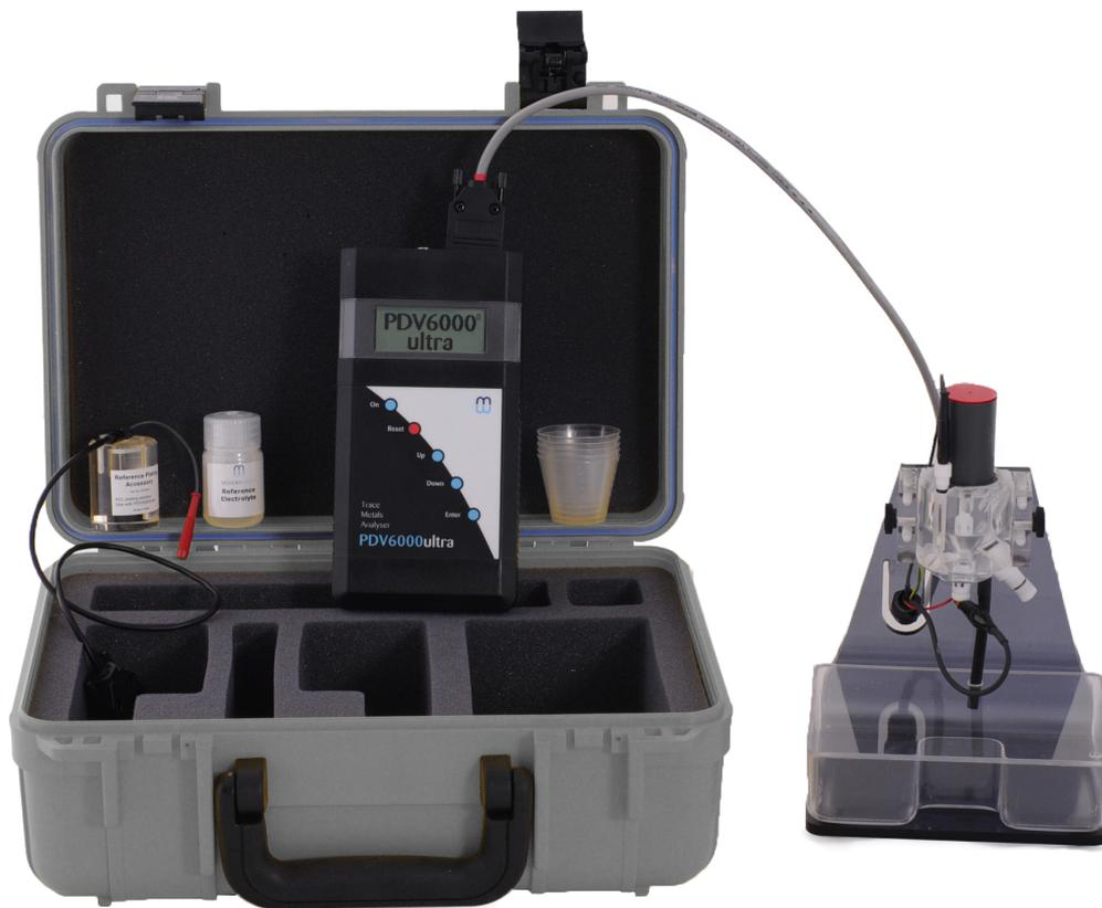
The PDV6000*ultra* has been upgraded to allow much improved stand-alone operation and an indication of blank and standard run performance. A larger screen allows simple voltammograms to be shown. The USB connector replaces the serial port. The upgraded product can be run either on 4 x 1.5V AA batteries, or from the mains using the standard 8 - 12V DC transformer.
